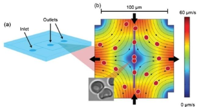
Device schematic and view of cross-junction, with cells entering and exiting
